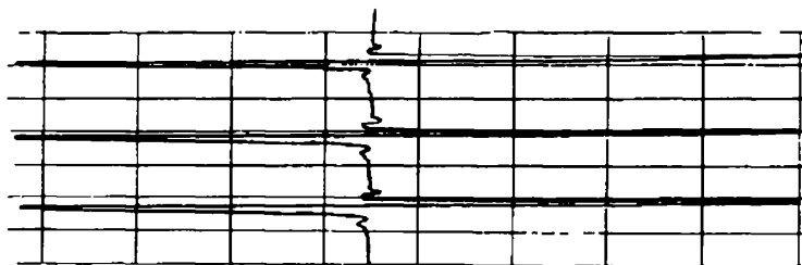
FIG. 2. ESR spectrum exhibited by a solution of 2,2,6,6-tetramethyl-4-piperidone nitrogen oxide in water.
